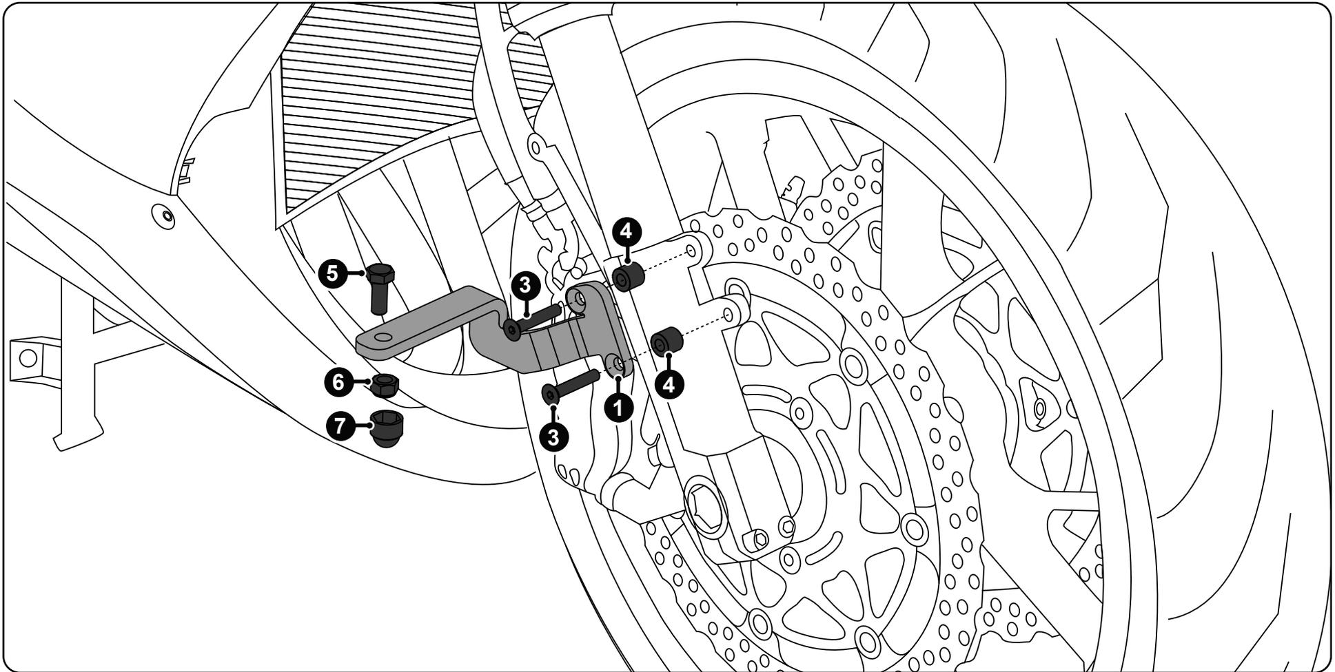
**Step One:** Remove the front fender to expose the mounting points illustrated above. Use the bolts (#3) and spacers (#4) to mount the left and right side brackets (#1 & #2) to the motorcycle using the OEM fender bracket as the backing plate. Use the remaining hardware, bolts (#5), Nuts (#6) and nut caps (#7) to mount the light pods to the brackets. Reinstall the front fender to the motorcycle.
