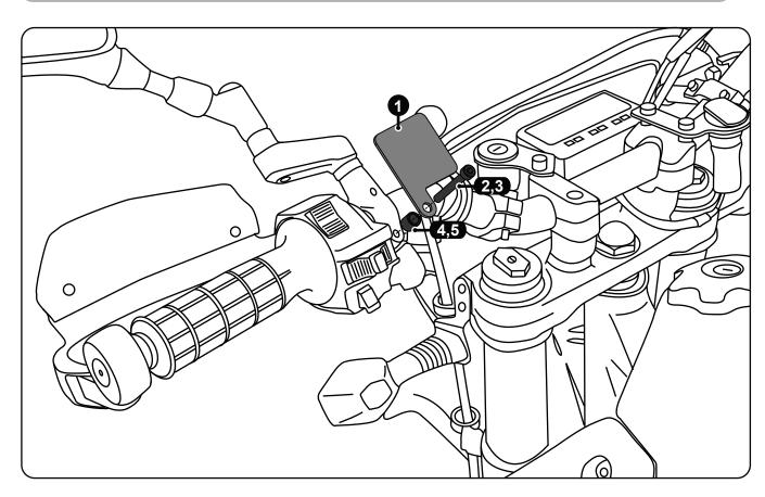
**Step One:** Attach the mounting bracket to the perch using the included bolts and spacers to obtain the proper thread length. The bracket may be mounted off either bolt on the perch and rotated in any direction to best suit your motorcycle.
