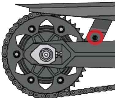
2. Using the M6 screw, washer and nyloc nut in this adapter kit - fix the dispenser plate from the main kit to the inside face of the swingarm through the chain guard mount.
