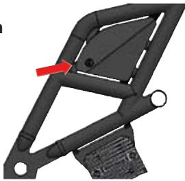
2. Locate the vacuum bung on the bottom of the airbox, in the middle of the bike.
