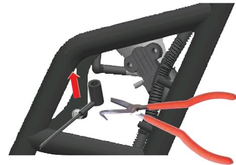
Use a downward pulling motion, do not use a sideways motion.
