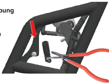
4. Push the black vacuum tubing from the kit into the damper elbow (SA-0103). Then firmly press the damper elbow onto the spigot on the airbox, until it can go no further.
