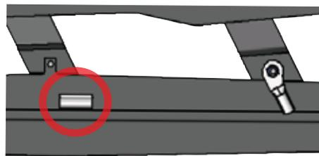
4. Secure the dispenser assembly (part 2) to the dispenser plate by clamping around the black nylon sleeve using the jubilee clip from the vSystem. Route the delivery tubing to the RMV taking care to avoid the chain.
