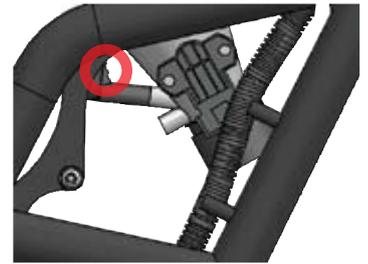
The end of the bung can just be seen behind the vacuum pipe from the throttle body to the airbox.
