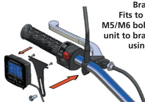
Bracket Mount. Fits to any existing M5/M6 bolt. Fit display unit to bracket (part 5) using M3 screws (part 16).
