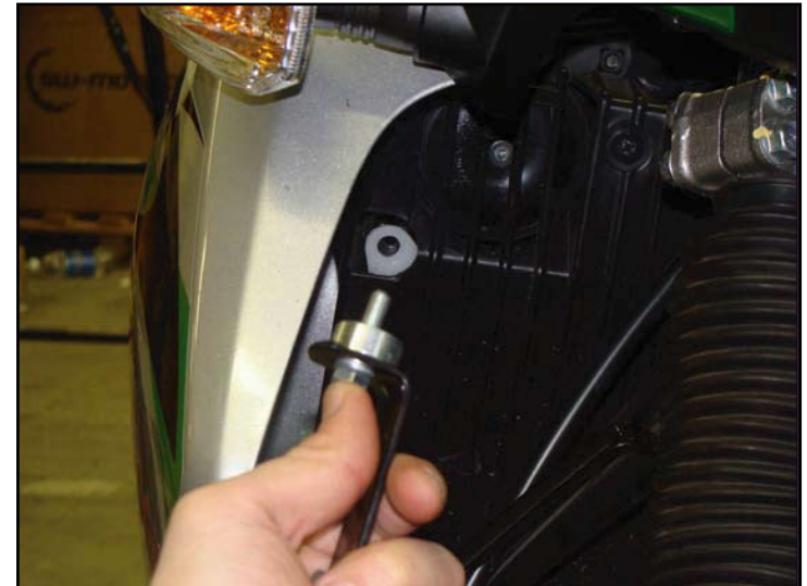
Attach the mounting bracket with the M6 screw provided. Place the 7mm spacer behind to the bracket.
