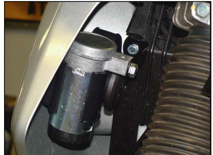
Mount the horn to the bracket using the hardware provided with the horn. Be sure to read all mounting instructions provided with the horn to ensure it is mounted at the right angle.
