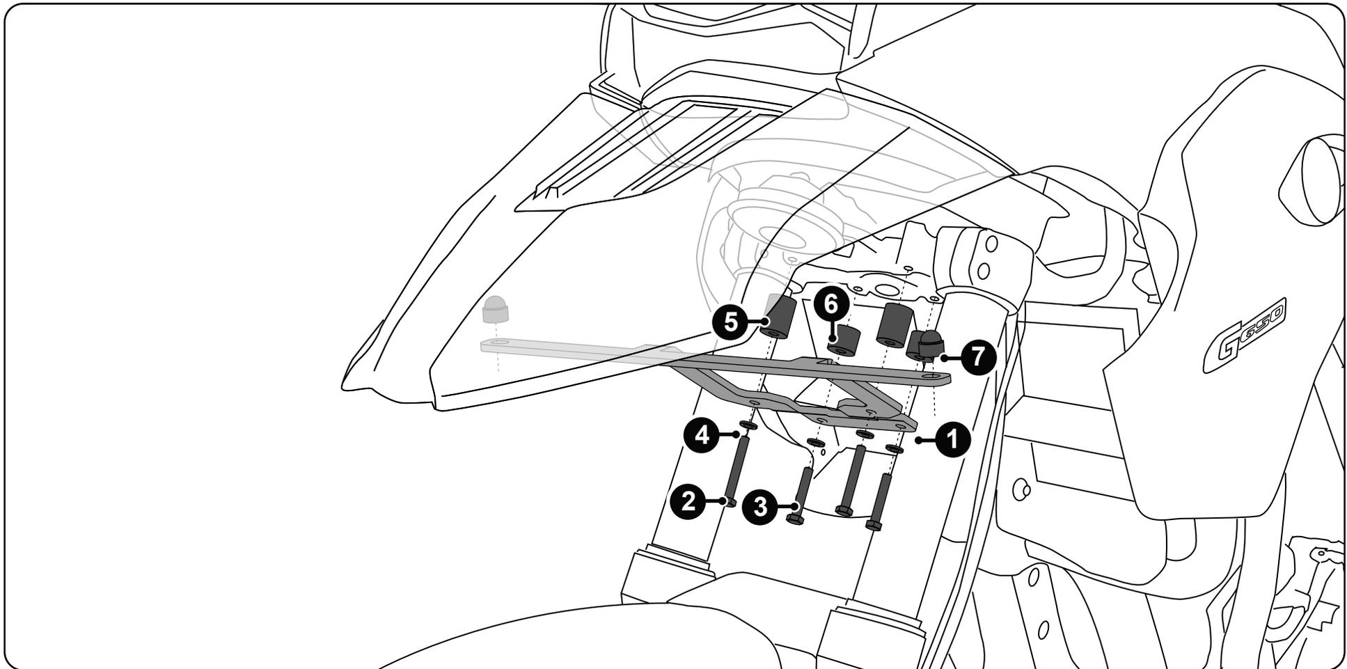
**Step One:** Remove the four bolts on the underside of the upper front fender. Use the supplied hardware to mount the light bracket to the motorcycle, the longer bolts (#2) and spacers (#5) mount into the holes towards the front end of the motorcycle. Use the supplied Nut Caps (#7) to cover the nut used to mount the light pods to the bracket.
