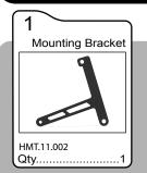
**Step One:** Remove the OEM lower left side radiator support bracket, be sure to keep all the harware as it will be used to reinstall the new bracket. Replace the bracket with the new horn mounting bracket as illustrated and reinstall the OEM hardware. Finally use the hardware supplied with your horn to bolt it to the bracket.
