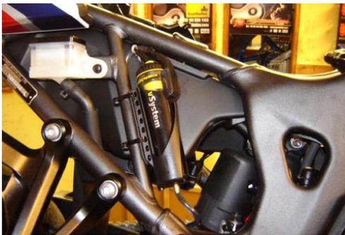
The dispenser can be held using the small dispenser plate and clip, secured by the rear sprocket guard bolt. The tip of the injector should lightly touch the face of the sprocket, with the slash cut facing outwards. The delivery tubing can be routed inside the swing arm to the rear of the suspension unit, and up to the RMV on the sub frame.
