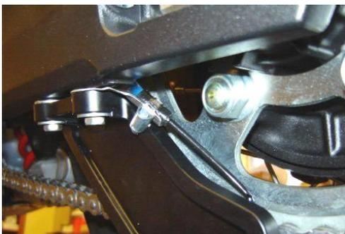
Once fitted, [fill and prime](#) the system and set the adjuster knob to 'prime'. Start the engine and turn the adjuster knob until a flow of between 1 and 2 drops per minute is achieved. Check the condition of your chain after a ride, and then adjust as required.
