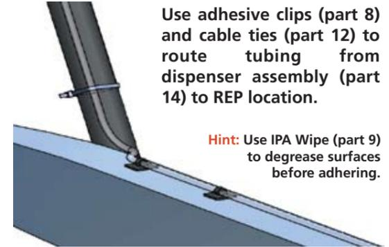
Use adhesive clips (part 8) and cable ties (part 12) to route tubing from dispenser assembly (part 14) to REP location.
