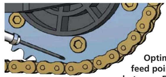
Optimum feed point is between 5 & 7 o'clock on the face of the rear sprocket.
