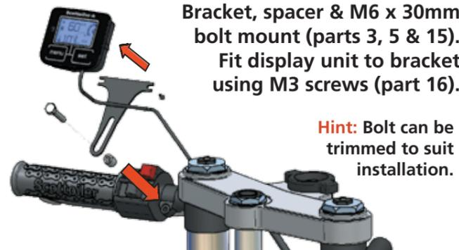
Bracket, spacer & M6 x 30mm bolt mount (parts 3, 5 & 15). Fit display unit to bracket using M3 screws (part 16).
