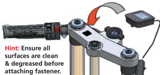
Hint: Ensure all surfaces are clean & degreased before attaching fastener.
